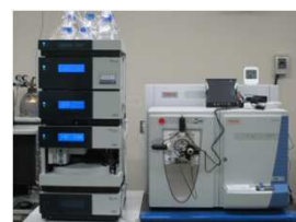
nanoLC-MS/MS System LC: UltiMate3000 RSLCnano MS: Orbitrap Elite
